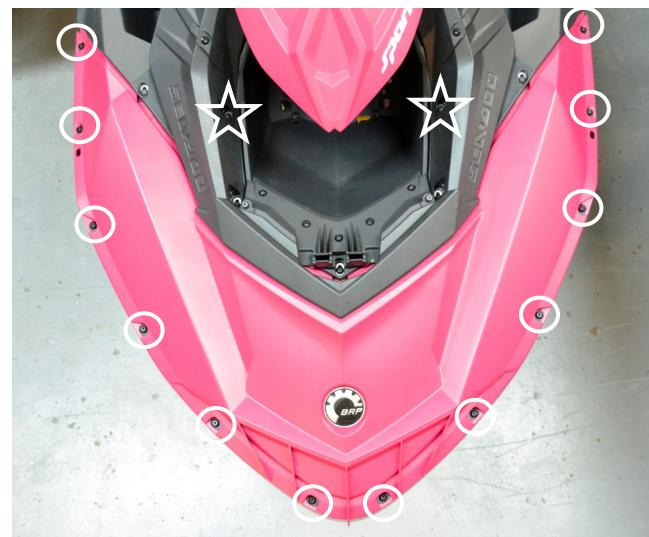
Discard plastic washers. Reinstall Torx bolts, upgraded washers in place of plastic washers, and nuts. **NOTE: Torque screws to 49 in•lb (5.5 N•m). DO NOT apply thread locking agent.**
