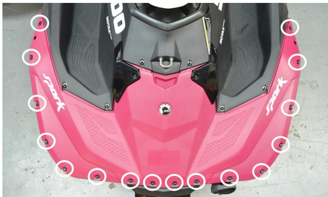
Discard plastic washers. Reinstall Torx screws with upgraded washers in place of plastic washers. **NOTE: Torque screws to 49 in•lb (5.5 N•m). DO NOT apply thread locking agent.**
